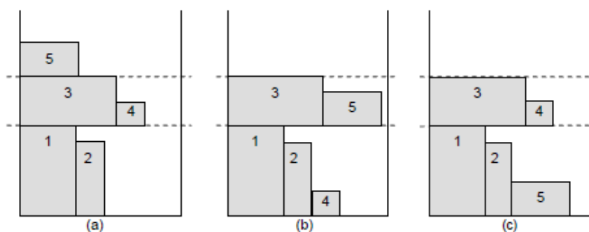
Slika 4-5: SH algoritam za 2SP (a) NFDH , (b) FFDH i (c) BFDH
